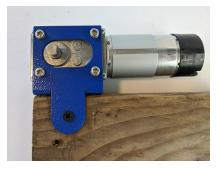
6. Attach E1 motor sprocket by inserting the E2 grub screw into the gear hole, aligning with the flat side of the motor shaft, and tightening with E5 Allen wrench to prevent slipping.
