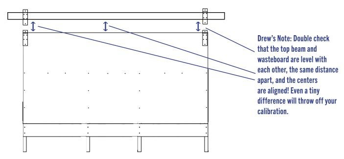
2. The material you are cutting will need to by clamped to the wasteboard stud mounts or screwed into the wasteboard. We recommend both clamping at the top and screwing in at the bottom to prevent warping.
