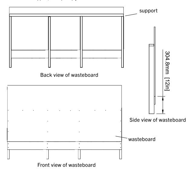
6. Two of the stud mounts will hold your wasteboard at the top corners, so it rests at a 15 degree angle when you're cutting (with the largest end closest to the ground). Find two studs in your wall that are 8' apart and mark them. Then, lean the wasteboard against the wall and align one of the studs close to the edge. Hold the stud mount between the wall and the leaning wasteboard and mark the top hole of the stud mount. Attach it to the stud in the wall using D2 screws.
